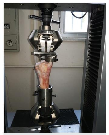
Figure 2. Application of tensile forces to the prepared samples
